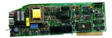
ProModem 1200A is a 1200/300 baud Hayes compatible auto-dial modem card that plugs directly into any expansion slot in the Apple II, II+, or IIe. All you have to do is plug it in and connect the telephone cord.
